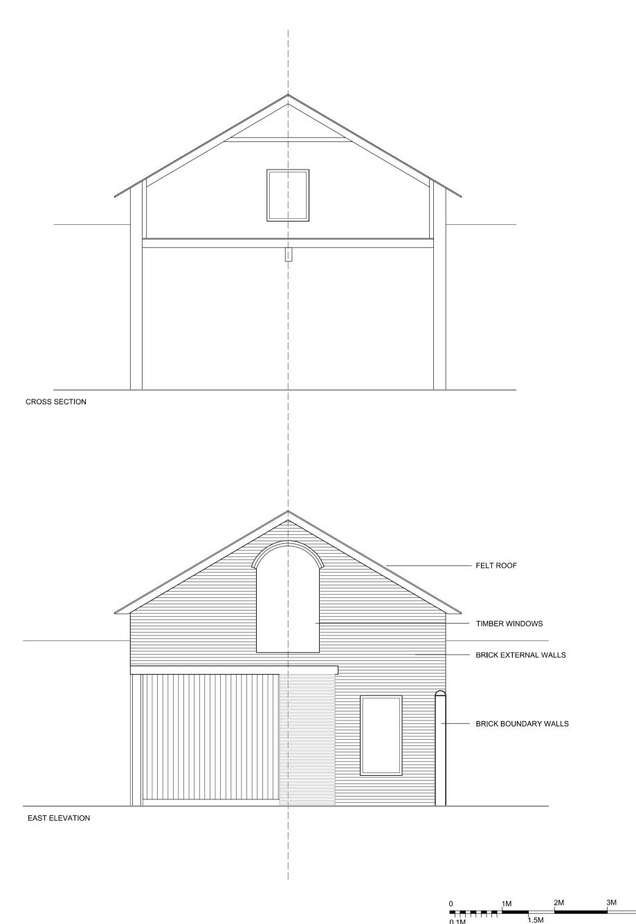
PL(060)013\_EXISTING EAST ELEVATION AND CROSS SECTION rev A SCALE 1:50@A3
